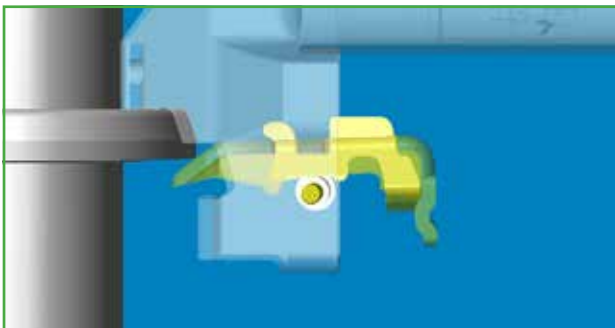
Figure 5 – Wedge Retainer with Plastic Tube (Contacting Ring)
