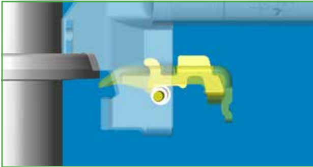
Figure 4 – Wedge Retainer with Plastic Tube (Disengaged)
