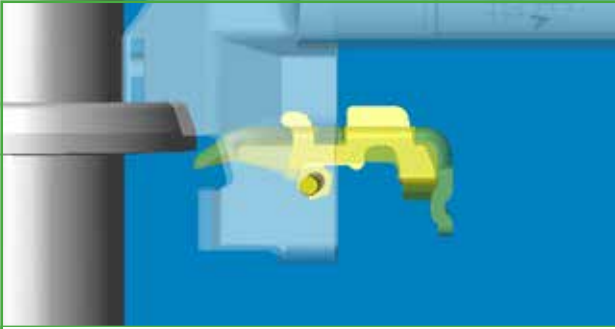
Figure 7 – Wedge Retainer without Plastic Tube (Disengaged)
