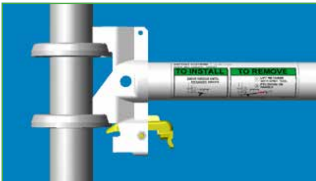
Figure 2 – Wedge Operation (Contacting Ring)
