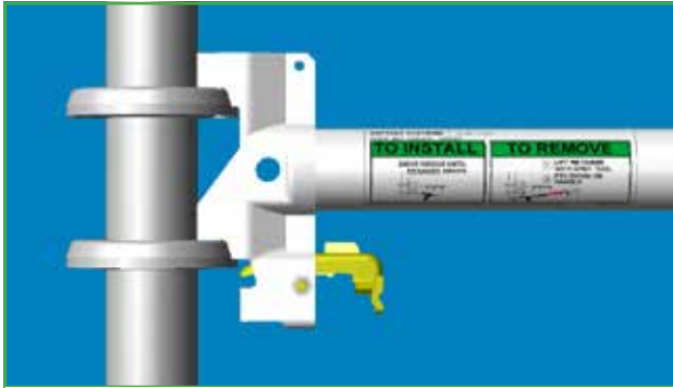
Figure 1 – Wedge Operation (Disengaged)
