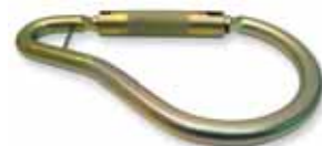
VSEP407 (TT) Alloy steel 2 3/4-in. opening 7,200-lbs. MBS
