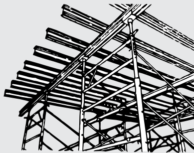
Safway® ALJ Aluminum beams can be used as both joists and stringers.
